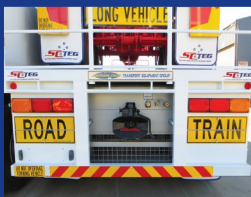
Road Train Coupling & Signage
